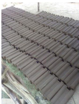
Figure 18: ISSBs produced by the Majengo RC CMF group (left) used in the construction of community facilities
